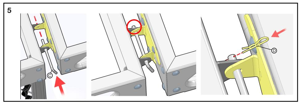
Connect the docks by sliding a Hinge Pin (C) into the hole between the hinges (See above). Slide the Hinge Pin (C) into place. Insert the Cotter Pin (D) into the hole at the end of the Hinge Pin (C). Do the same for both hinge assemblies on the opposite side of both docks.
