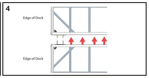
Once Hinges (A) on both docks are assembled pull both docks close to each other. Place the docks so the edges of both docks are aligned with one another. Aligning the hinges on either side of the docks so they fit into each other. Ensure that the holes between both hinges line up with one another. Do the same for the hinges on the opposite side of both docks.
