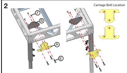
On the dock connect the Hinge (A) to the Triangle Plate (B) using Carriage Bolts (E) and , K-Lock Nuts (F) as shown. Using a hinge from the second pair follow this step for the opposite side of the dock. PLEASE NOTE: The decking has been removed from images shown to better illustrate installation.
